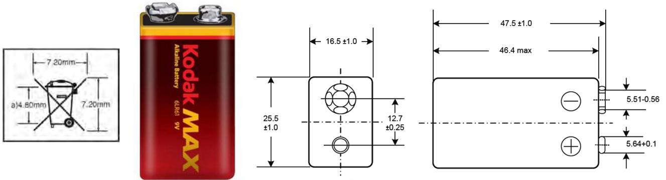
Dimensions are in millimeters and include label.
